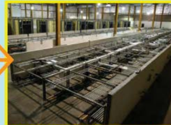
MEP corridor racks lined in the prefabrication warehouse
