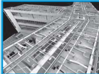
Building Information Model (BIM) of the MEP corridor racks
